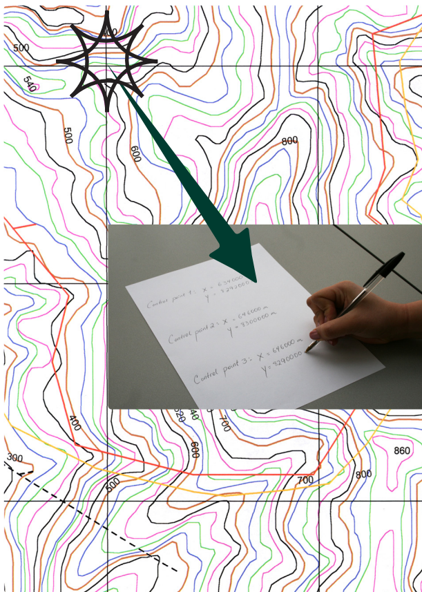
Figure 67. Control point coordinates are recoded from the base map
