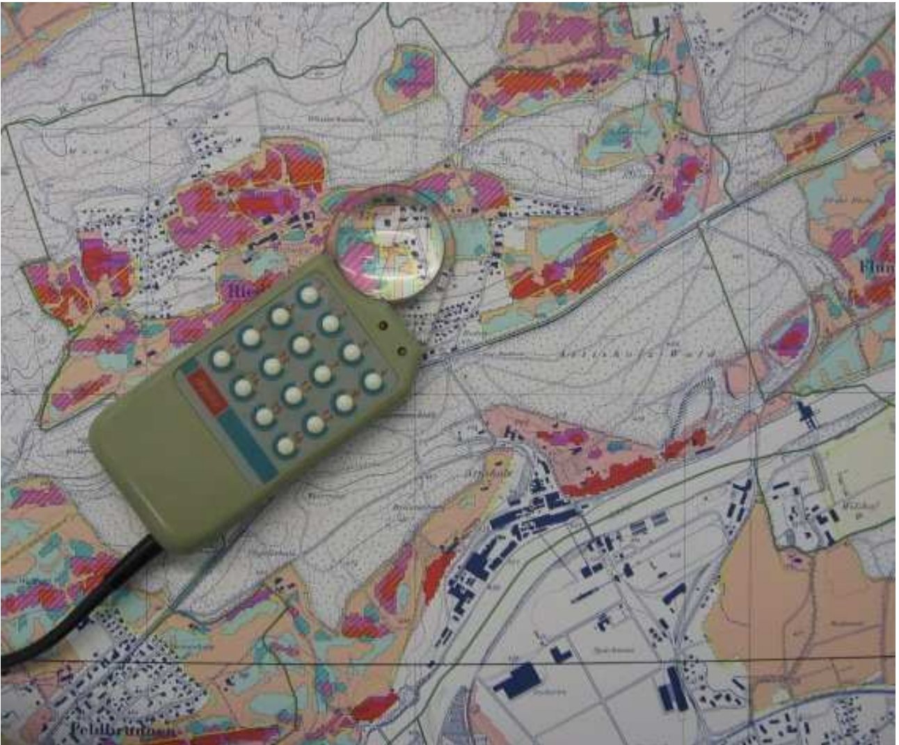
Figure 39: A digitising table and puck are used by GIS professionals when they want to digitise features from existing maps.
