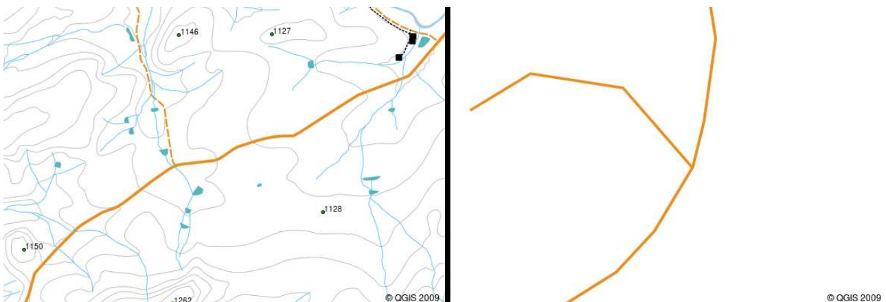
Figure 12: Polylines viewed at a smaller scale (1:20 000 to the left) may appear smooth and curved. When zoomed in to a larger scale (1:500 to the right) polylines may look very angular.
