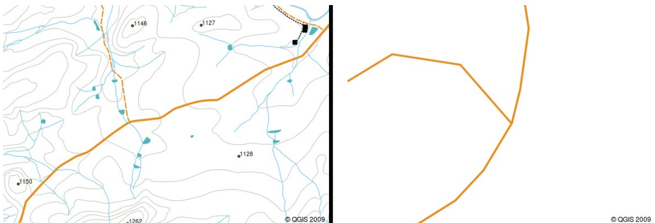
Illustration 19: Polylines viewed at a smaller scale (1:20 000 to the left) may appear smooth and curved. When zoomed in to a larger scale (1:500 to the right) polylines may look very angular.
